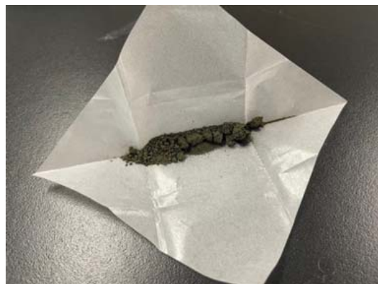
Fig.3 Produced titanium sulfide powder as intermediate material using coffee husk as biomass fuel / コーヒー殻を用いて作製した硫化チタン粉末
